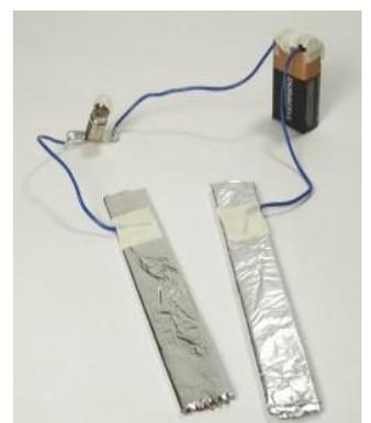
5. Use the third piece of wire to connect the negative terminal of the battery with the other electrode.
